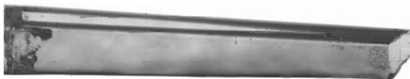
Figure 9. Absorption contrast—presence of Pb inclusions in the bottom region (darker colour, left-hand side).
